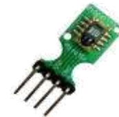
Gambar 3. Sensor SHT11 (Sumber: Lau, 2017)
